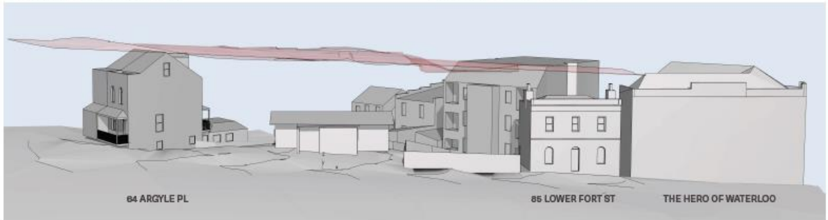
12m height plane corresponds to the ridge heights of 64 Argyle Place and The Hero of Waterloo pub on the corner
